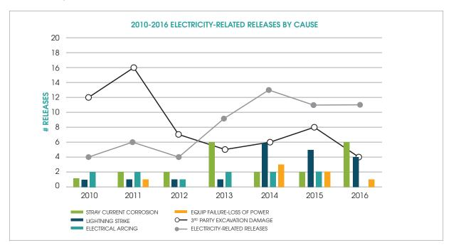
The leading causes of electrical related releases are stray current corrosion and lighting strikes, which affect onshore pipelines and facilities most frequently.
